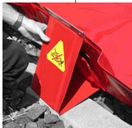
Correct anchoring of the side support
