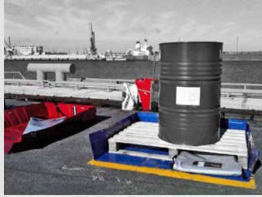
The corners are not sealed and so the tarp can easily fold around the pallet
