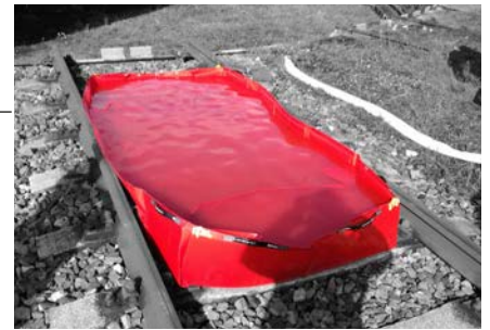
There are two ways to place the tank under a train or other track vehicle: across the rails or along them into the inner space between the rails. Both ways passed very strict testing.
