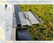
Tubebarrier uses universal ground anchors which function on nearly every surface. Each meter of Tubebarrier uses a kit containing 2 ground anchors, including12 wedges, 4 pins and 4 wood wire bolts. This kit is delivered as a single item. And weighs in total + - 2kg per meter. The components are made of aluminum.
